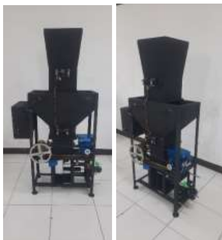
Figure 3 Smart Waste Processing Machine Prototype for Sorting, Shredding, and Compaction
