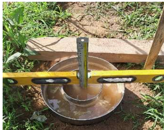
Figure 1. Double ring infiltrometer
